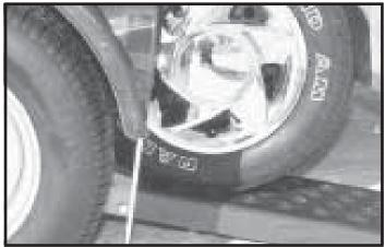
**Step 6.** With someone safely guiding you, slowly drive vehicle onto platform **FRONT FORWARD**. (Any vehicle mounted on tow dolly must be mounted with front of the vehicle facing forward.) Drive the car forward until the tires touch the ramps. Make sure the tire is aligned to ascend onto the ramps.
